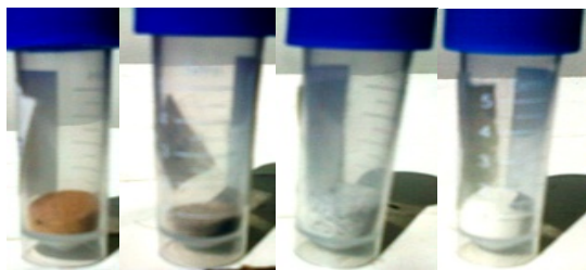
Fig. 1. Samples A, B, C & D were processed at 350°C, 500°C, 650°C & 900°C in a furnace for an hour.
